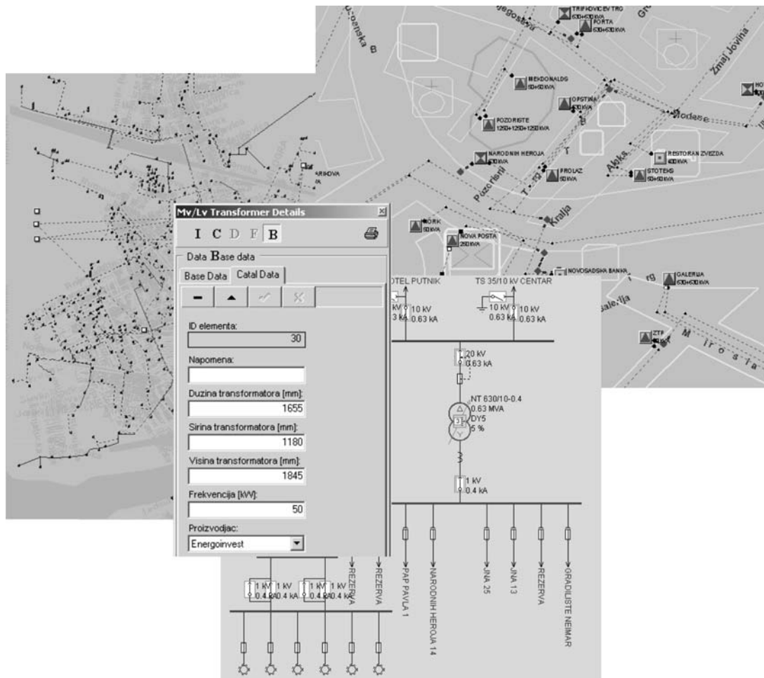
Figure 3 – Substations data overview.
